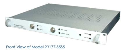
This 2x2 switch operates over the DC to 6GHz frequency range. It is designed to be controlled from the external alarm contacts of devices such as modulators. The unit can be controlled locally via front panel push buttons and remotely via an external alarm contact on the rear panel.
